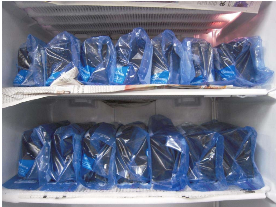
Figure 4-11 Oil sand blocks stored in air-tight packing in a cold environment
