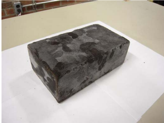
Figure 4-10 A frozen oil sand block
